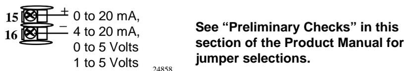
**Figure 2-8 Input 2 Connections**
